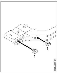
► Insert square nuts (1) in the barrier bar (2) – the holes must line up
